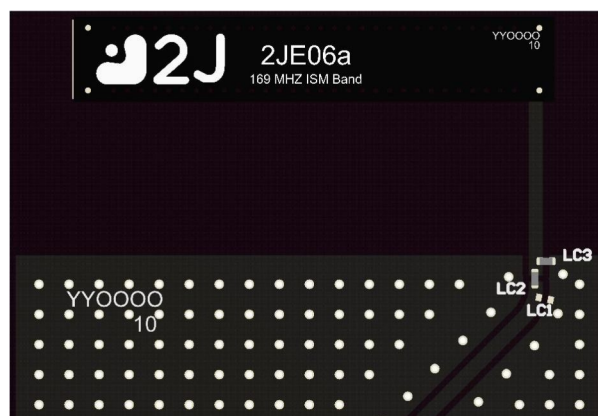
3D View of matching components and recommended values (LC1 = OPEN, LC2=3.3pF, LC3= 180nH)
