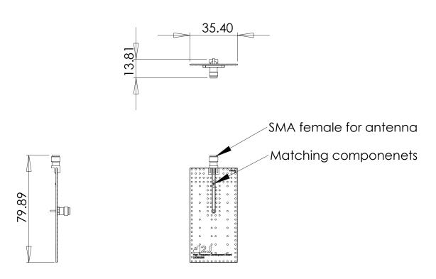
This development board is suitable for finding best matching componnets for high frequency antennas and test high frequency antenna as ground size is similar to most of the existing devices on market.
