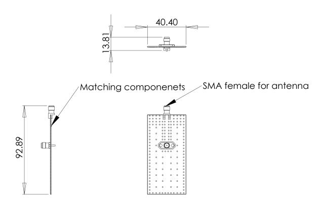
This development board is suitable for finding best matching componnets for GNSS antennas and test GNSS antenna as ground size is similar to most of the existing devices on market.
