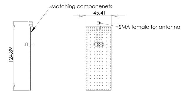
For matching componenets can be used up to 3 componenets in Phi network. But in default is used just 0R resistor for connecting input port with output port.
